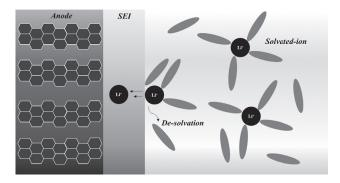
Figure 1-2. Reaction mechanism on the anode of lithium-ion rechargeable batteries
