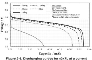
Figure 2-6. Discharging curves for ∳3x7L at a current value of 1C for different ambient temperatures
