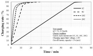
Figure 2-3. Relationship between charging time and charging rate of  $\varphi 3x7L$  at different charging current rates
