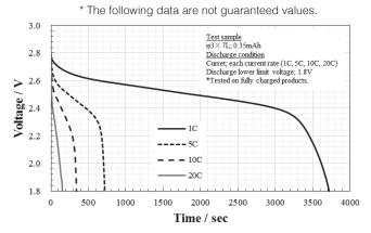
Figure 3-2. Relationship between discharging current value and discharging time for  $\phi$ 3x7L
