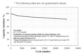
Figure 4-1. Rate of change in capacity of  $\phi$ 3x7L during charge/ discharge cycle test at current value equivalent to 10C
