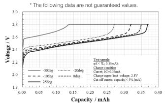
Figure 2-5. Charging curves for  $\phi$ 3x7 at a current value of 1C for different ambient temperatures
