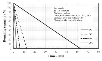
Figure 2-4. Relationship between discharging time and remaining capacity of  $\phi$ 3x7L at different discharging current rates
