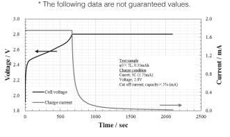
Figure 3-1. Constant current-constant voltage charging curve for  $\phi$ 3x7L
