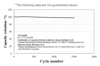
Figure 2-7. Capacity retention rate versus number of charge/discharge cycles when  $\phi$ 3x7L charged to 3.3V
