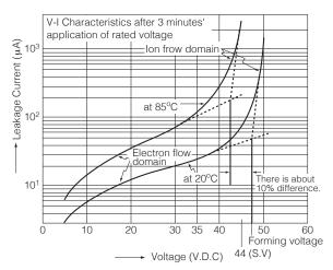
Fig. 2-4 V-I Characteristics (ex. Rated at 35V)
