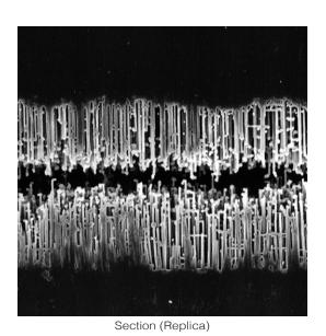
Photo 1-2 Surface and section photo of etched aluminum foil for middle / high voltage capacitors.
