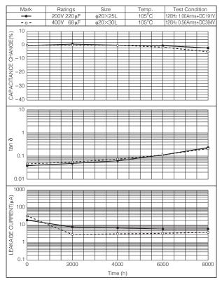
Fig. 2 - 13 High Temperature Life Evaluation Test
