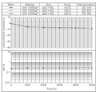
Fig. 2-16 High Temp. Evaluation Test
