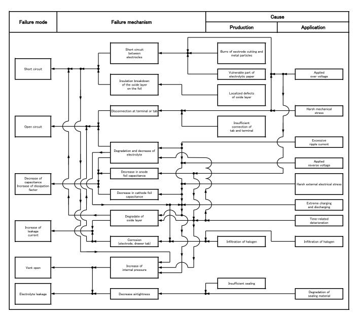
Fig. 2-1 Analysis of Failure Mode
