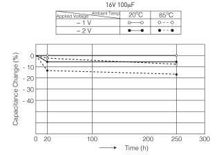
Fig. 2-3 Capacitance vs. Reverse Voltage Characteristics
