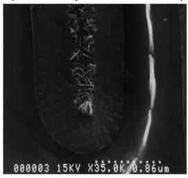
Photo 1-4 Enlarged photo of middle / high voltage formed foil. (State of oxide layer formed in a pit)
