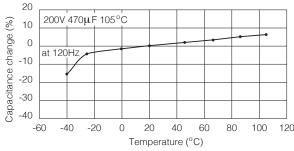
Fig. 1 - 9 Capacitance vs. Temperature Characteristics
