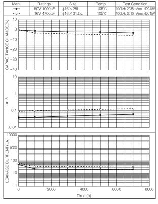
Fig. 2-14 High Temperature Life Evaluation Test
