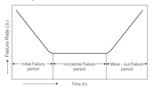
Fig. 2 - 11 Failure Rate Curve (Bathtub Curve)
