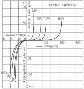
Fig. 2 - 2 V - I Characteristics (Voltage - Current Characteristics)
