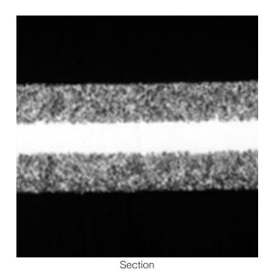
Photo 1-1 Surface and section photo of etched aluminum foil for low voltage capacitors.
