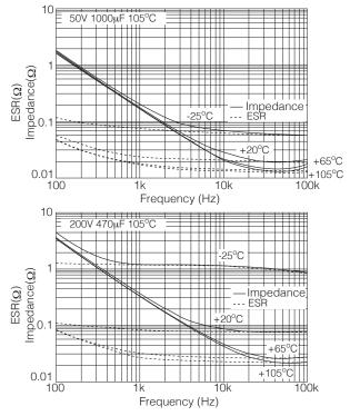
Fig. 1 - 11 Impedance, ESR vs. Frequency Characteristics
