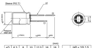
(¢D < 10) 1.5 φD 6.3 8 12.5 10 16 18 α (¢D ≧10) 2.0 Ρ 2.5 3.5 5.0 5.0 7.5 7.5 0.6\* 0.6\* φd 0.5 0.6 0.8 0.8 % In case L>25 for the  $\phi$ 10 and  $\phi$ 12.5 dia unit, lead dia  $\phi$ d=0.8
