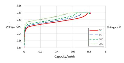
Charge : CC-CV 1C, 2.8V, cut-off 0.05C at 25°C
