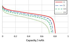
Charge : CC-CV 1C, 2.8V, cut-off 0.05C at 25°C
