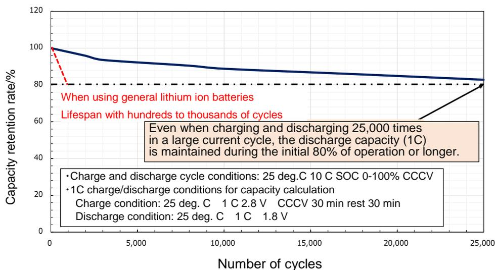
Figure 2: Charge and discharge cycle characteristics
